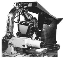
The AC-130U Gunship 25mm Linear Linkless™ ammunition storage and handling system, with a capacity of 3,000 rounds, represents the largest Linear Linkless™ system ever produced.
