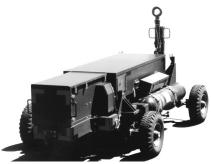
The Storage Container Assembly stores rounds in a serpentine fashion across three bays, using Parker Meggitt Defense Systems' Division innovative and highly reliable Linear Linkless<sup>™</sup> chain ladder system to provide 100% round control at all times with a reliability in excess of 200,000 mean-rounds-between-failure.
