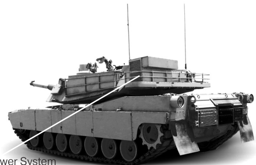
Auxiliary Cooling and Power System
