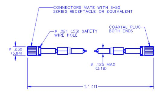
**LENGTH TOLERANCE TABULATION:** Standard cable lengths in inches: 36, 60,120
