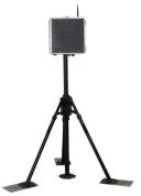
and a WLAN data link. Projectile data captured by the radar is stored locally. Processed data can be transmitted over the data link for remote storage and additional post processing.
