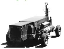
The Storage Container Assembly stores rounds in a serpentine fashion across three bays, using Meggitt Defense Systems' innovative and highly reliable Linear Linkless™ chain ladder system to provide 100% round control at all times with a reliability in excess of 200,000 mean-rounds-between-failure.
