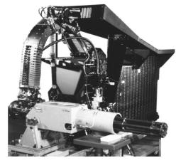
The AC-130U Gunship 25mm Linear Linkless™ ammunition storage and handling system, with a capacity of 3,000 rounds, represents the largest Linear Linkless™ system ever produced.
