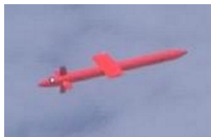
Target released and executes pre-programmed, multiple way point GPS navigation during free flight
