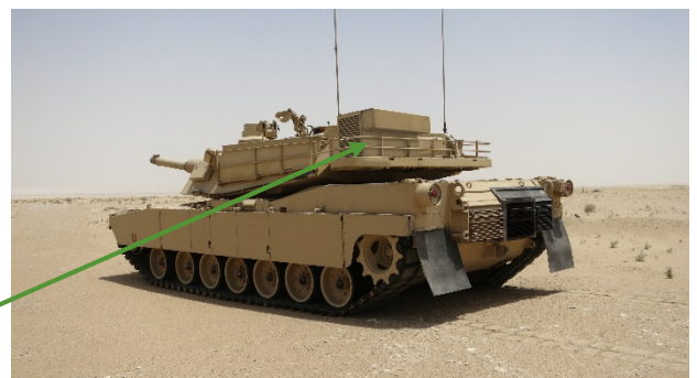
Auxiliary Cooling and Power Unit
