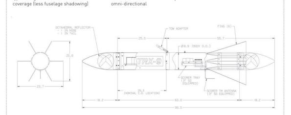
octahedral retroreflector array (forward and aft)
