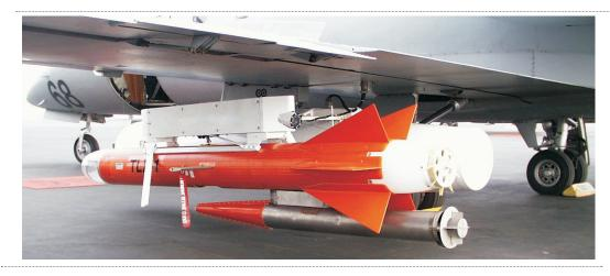
The main feature for the TLX target is the ability, via use of sophisticated, computer-controlled design, to realistically simulate an extremely low altitude missile threat. This is accomplished with a height-keeping flight profile which positions the TLX at any desired mission altitude from 20-500 feet while providing constant altitude feedback to the towing aircraft via telemetry link.
