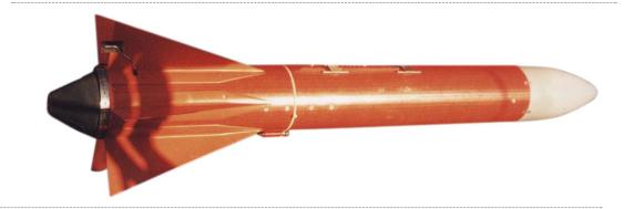
The TIX Infrared Augmented Tow Target is designed for use with weapon systems or trackers that employ heat seeking guidance technology. An infrared emitting propane burner which operates at approximately 1135C, provides the infrared output.
