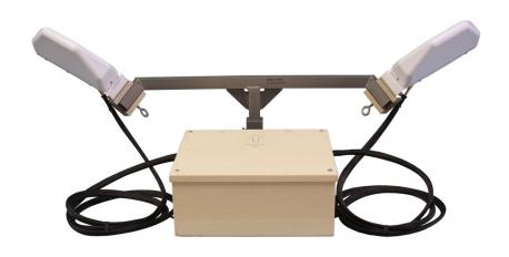
The Round Identification and Location System (RILS) is a standalone Doppler radar scoring system. The heart of RILS is the Non-Contact Hit Sensor (NCHS) that provides location and identification of projectile types along with velocity and angle of approach in realtime. Hit data from the NCHS is uploaded to the laptop ground station through a WLAN.
