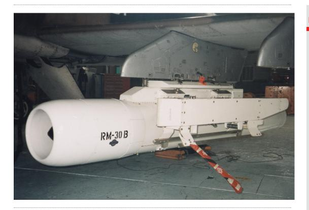
The RM-30B Reeling Machine-Launcher was developed to operate on modern fighter jet aircraft for the purpose of supporting both the short tow gunnery and long tow missile target missions using one reeling machine configuration. The machine is a derivative of the RM-30A and RMK-35 machines, it has the load capacity of the RMK-35, the towline capacity of the RM-30A, and is powered by the higher output turbine of the RM-30A1.
