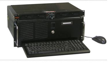
The AN/GSQ-228A operates in conjunction with the Meggitt Defense Systems, Inc. [MDSI] AN/DSQ-50A scalar scoring sensor to produce scalar scores. It also operates with other MDSI sensors such as the VDOPS vector scoring sensor to produce vector scores with weapon attitude information. It is the standard US Navy score processor and is deployed on all US Navy test and evaluation ranges.
