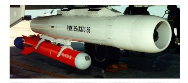
Developed in the early 1980s to replace the TDU-19B Dart target and interim A/A37U-33 (Secapem 90-6), the AGTS-36 system meets all aerial gunnery training requirements of a modern fighter aircraft.
